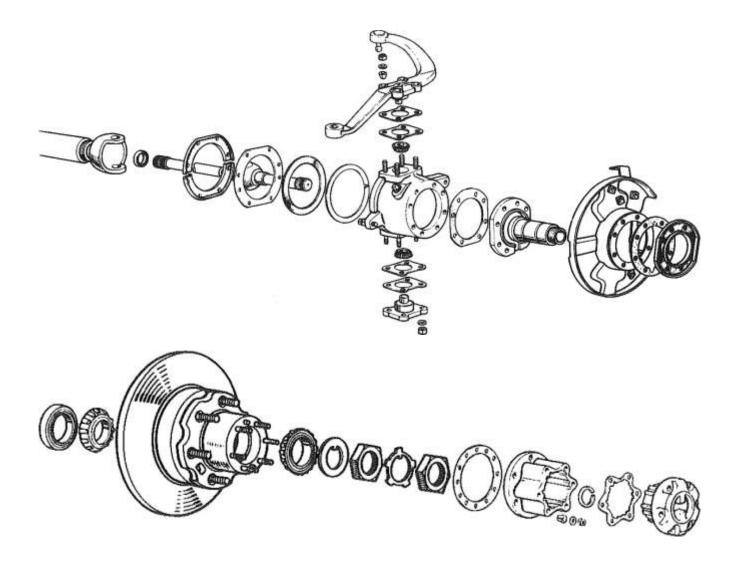
**Please Note.** To remove the hub stud and cone washers use a tapered punch or aluminium or brass drift on the end of the studs, the cone washers will release on impact.
