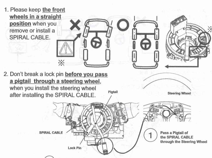
2 Break a Lock Pin of the SPIRAL CABLE.
